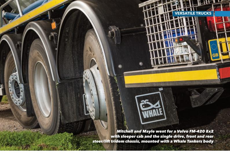
the tridem concept having witnessed its capabilities on a neighbour's hookloader. "We did our research online and it was clearly capable of getting into tight spaces," he says. "Also, the rear bogie has a 24-tonne capacity, which is good for us."
