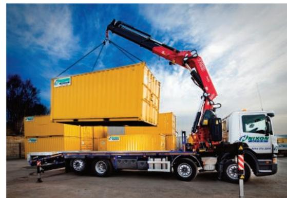
***“Where space is limited and legs can only be deployed so far, the control system can respond dynamically to the truck counterbalance weight, rather than restricting loader performance according to leg deployment alone”***
