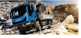
The new variant's Euro 6 package includes a four-cylinder, 3.0-litre heavyduty common rail engine delivering 170bhp and 400Nm of torque. The sixspeed overdrive gearbox is coupled to a central transfer case with four low ranges, yielding 24 ratios in all. Such a spec, and a vast choice of PTOs (power takeoffs) probably allows it to sit beside the Unimog without feeling too small.
