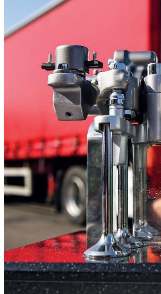
When the piston reaches top dead centre, the accumulated compressed air in the cylinder is vented, before it can act like a spring to drive the piston back down. By doing this the engine slows the vehicle, and also acts as an air compressor.
