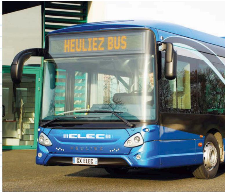
tailpipe emissions provided in operation by the full-electric Series-EV comes to the fore. Its direct drive DC traction motor takes power at high voltages (500-750V) from a battery pack, via a propulsion control system, turning the driven wheels via driveshaft and differential. Even though it contains no engine or generator (unlike the Series-ER), the system still handles bi-directional energy
