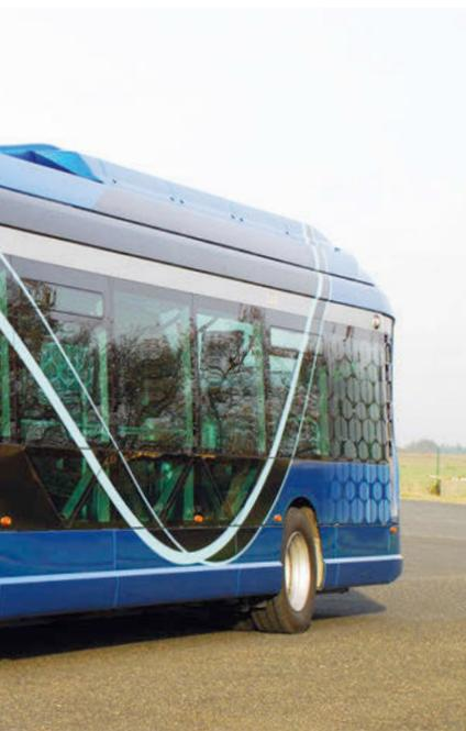
continuous at 1,100rpm), fitted to 360kWh batteries mounted in a 12m chassis from Heuliez Bus. In Mulhouse, the five steel chassis/composite body buses were equipped with NMC batteries from Forsee Power. Fitted with air conditioning, heating and an integrated access ramp, they accommodate up to 90 passengers with two wheelchair spaces.
