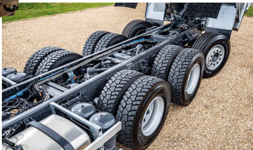
some competitors', is well-protected with steering arms tucked out of harm's way. This, along with the position of the rear air bags, makes it possible to tip into an asphalt paving machine without fouling, an important consideration for tippers.
