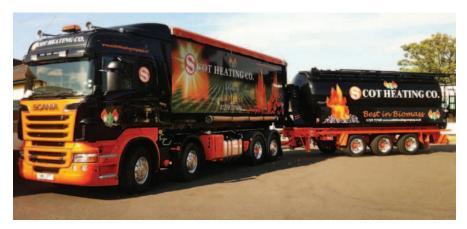
Scot Heating has taken delivery of a specialised Scania R 500 LB8x2\*6HSA drawbar unit, with triple steer axles.
