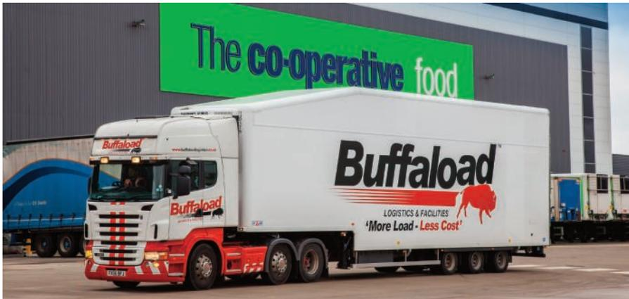
With 44-pallet capacity, these Gray & Adams double-deck semi-trailers can provide up to 66% more volume than conventional temperature-controlled trailers
