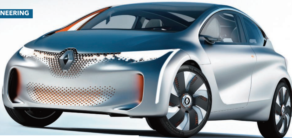
The EOLAB concept car exhibited by Renault at the Paris Motor Show last October. Features include ultra-thin 3mm windscreen glass, offering a 2.6kg weight saving as part of a package of measures that make EOLAB 400kg lighter than the equivalent Clio. It's only a matter of time...
