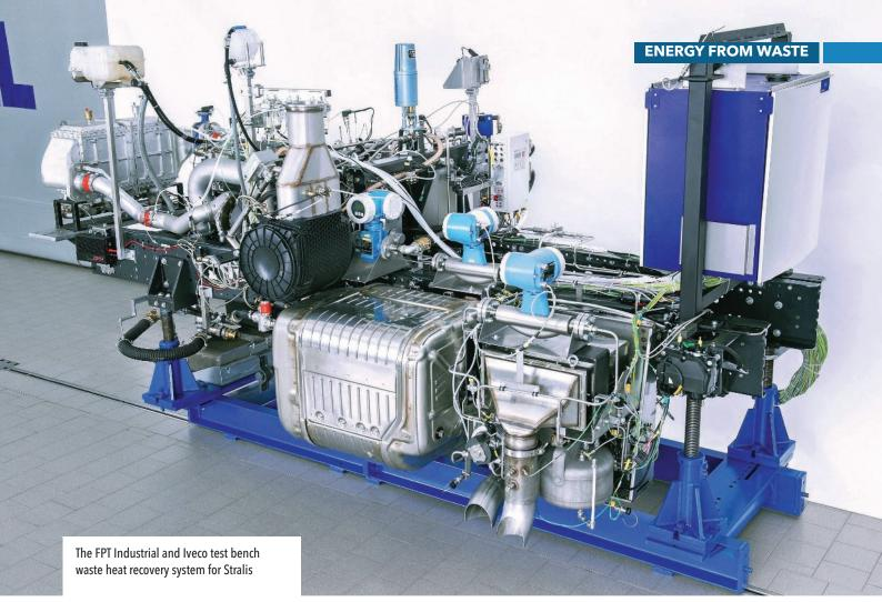
rowing numbers of truck and engine makers have been citing waste heat recovery (WHR) as likely to play a key part in raising diesel engine brake thermal-efficiency (BTE). They also point to WHR's ability to improve fuel economy and hence also cut greenhouse gas emissions. Compared with many other future truck predictions, this re-engineering approach appears to have legs.
