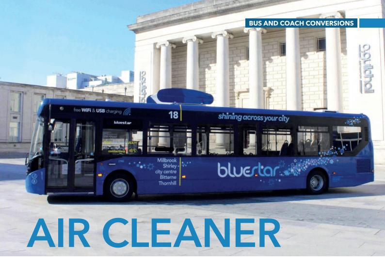
ince the end of September, one of the Euro VI diesel-powered single-deckers running out of Go-Ahead's Bluestar Eastleigh (Southampton) depot has been carrying a 600mm-high backpack. This 25kg proof-of-concept unit consists of filter media and an electric fan to pull particulate matter, PM, out of the air and trap it on the filter, which is said to catch 99.5% of particles up to 10 micron in size.
