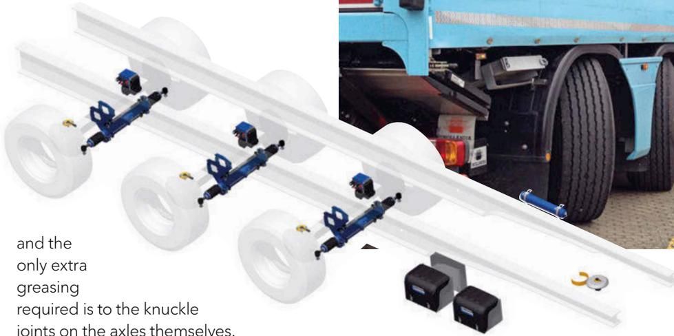
and the only extra greasing required is to the knuckle joints on the axles themselves.
