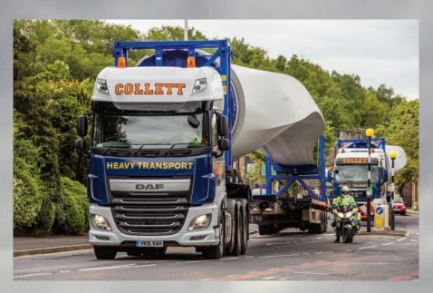
Sliding under the trailer, Collett's driver commented that putting 20 tonnes on the fifth wheel made little impact on the springs, which have a seven-leaf trapezium layout with 29mm leaves. As for the choice of manual gearbox (16 speeds in the FTM), Jack Collett, renewables division manager and manager for this project, is pragmatic. "We use manual and automated transmissions across the fleet, with no special preference. If our drivers have a leaning, it would be towards a manual box."
